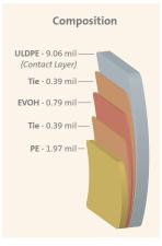
Single-ply multilayer structure with inert PE fluid contact layer. Film is animal-free—Rocker cell culture bags.
