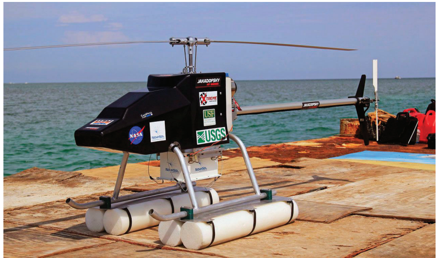
FIGURE 2. VisionII UAV with SHARK system, including the monolithic visNIR HSI sensor, flies from a deployment barge to conduct studies of Florida coastal waters.
