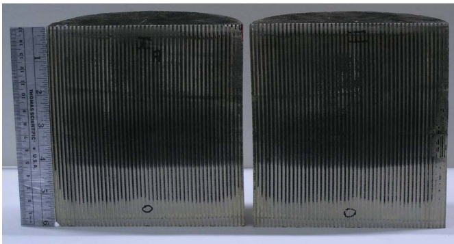
Figure 23. Pictures of filter 5 after 120,000km of operation and several hundred regenerations. Picture shows the inside of the zone-coated filter after de-canning and cutting into two halves. Filter inlet is at the top.
